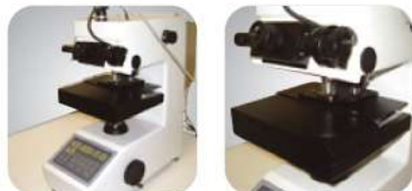
Step motor driven automatic X-Y stage of MH-6S
