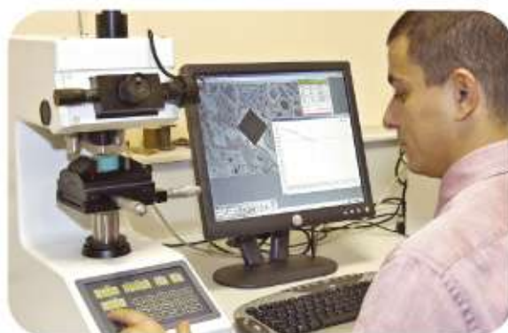
VMS 2000 can be connected to MH and VH hardness testers for semi-automatic operation and "Case Depth" hardness measurement at an affordable price/performance ratio.
