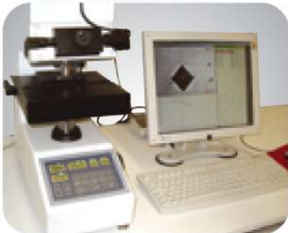
MH-6S Fully Automatic Microhardness Testing System with Autofocus and Autoreading for serial "Case Depth" hardness measurements.
